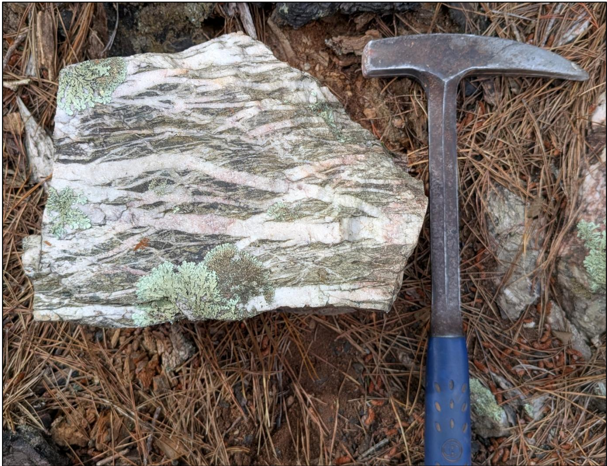
Figure 1. Stockwork quartz veining at the AC Prospect. Sample 9332-103 collected
