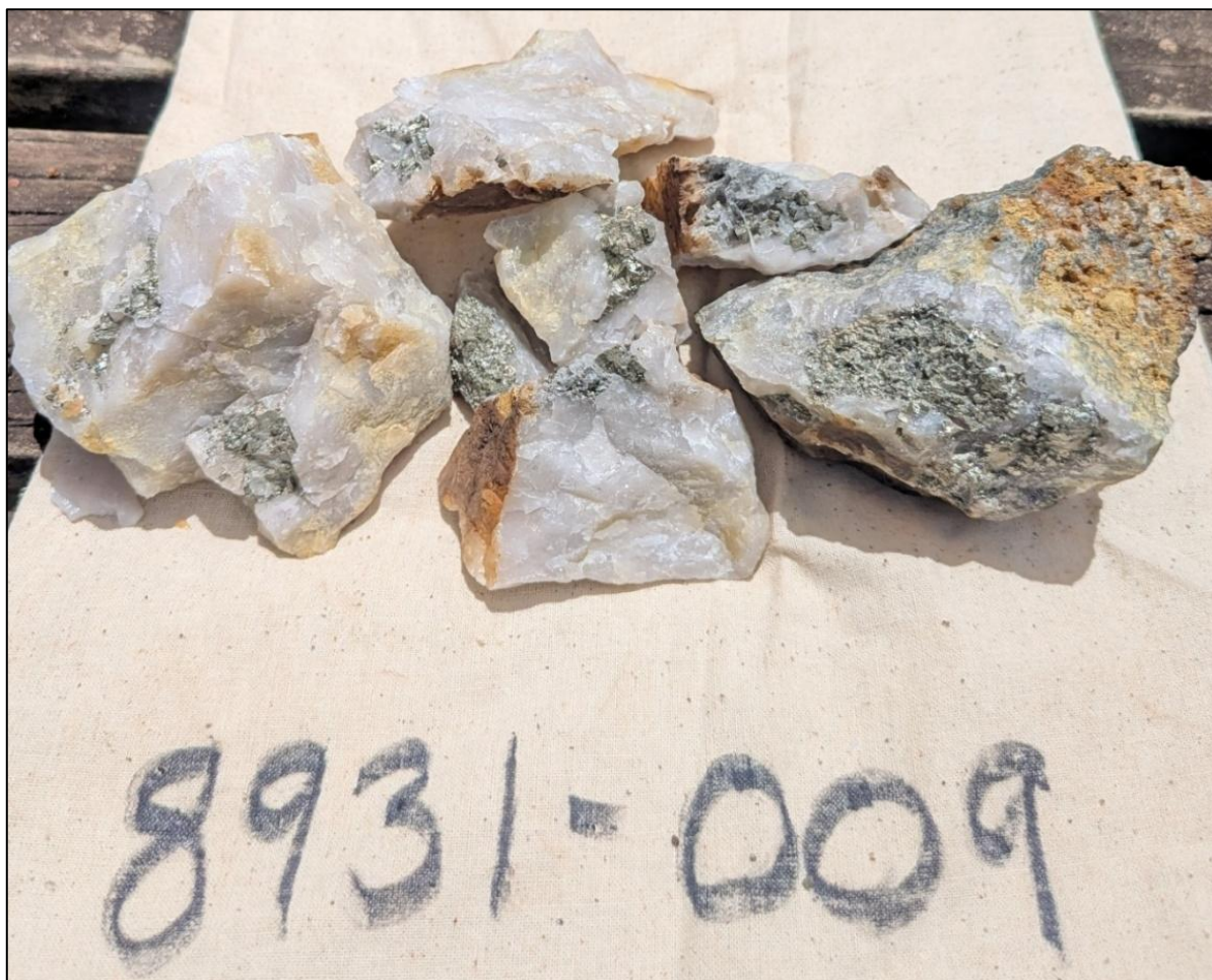
Figure 3. Rock chip sample 8931-009: Quartz-pyrite veining from the Undoo Creek prospect - 5.42g/t Au
