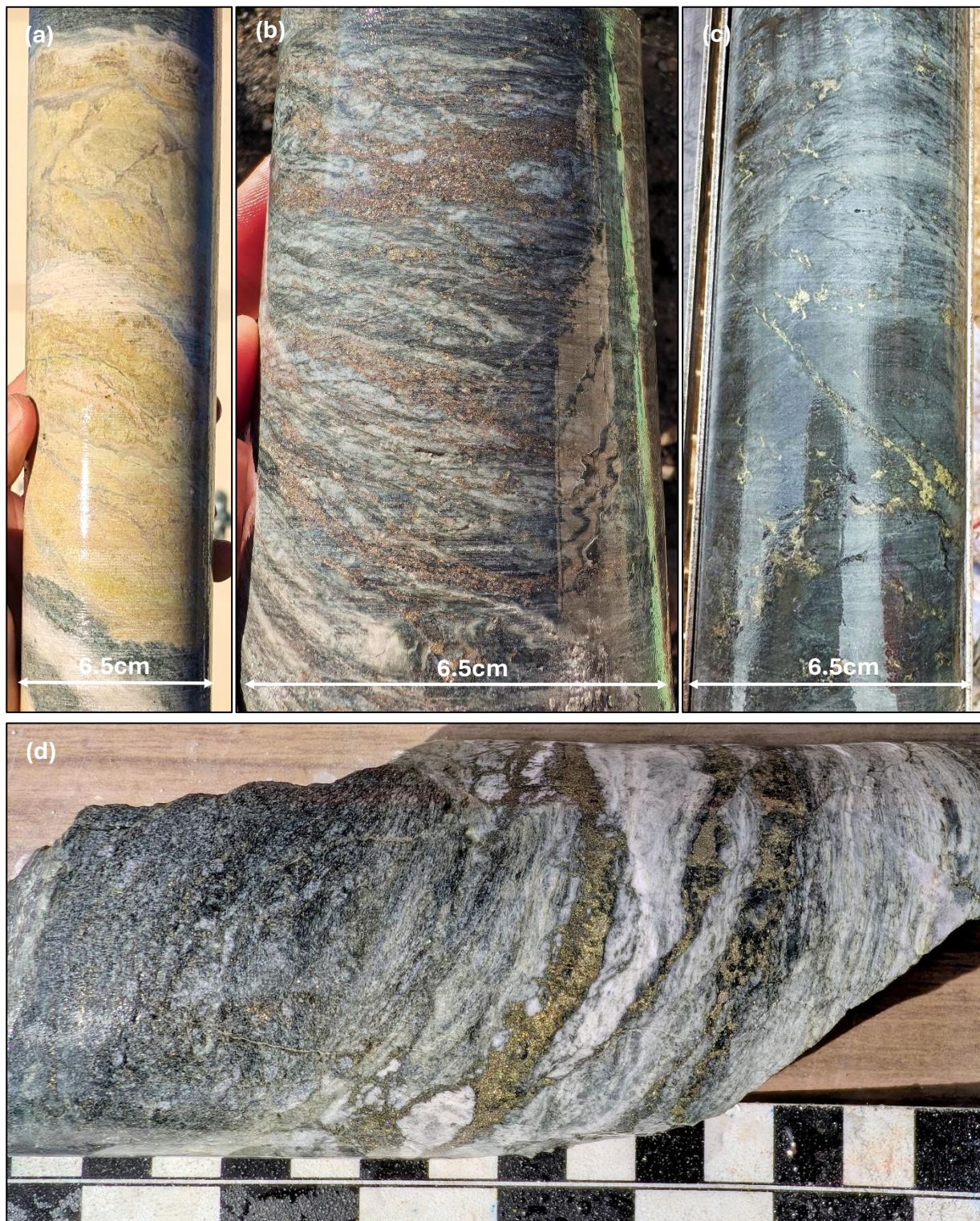
Figure 2. (a) Intense sericite-silica-carbonate-chlorite alteration of volcaniclastic sandstone in BLRCDD001, 77.3m. (b) Strong sphalerite-pyrite-galena mineralisation in BLRCDD001, 84.5m. (c) Fracture-fill chalcopyrite-pyrite mineralisation in chlorite altered sediments in BLRCDD001, 105.7m. (d) chalcopyrite-pyrite veining in volcaniclastic sandstone in BLRCDD002, 164.8m. Visual estimate only; assays pending. Refer to Table 2 for visual sulphide estimates and cautionary statement.
