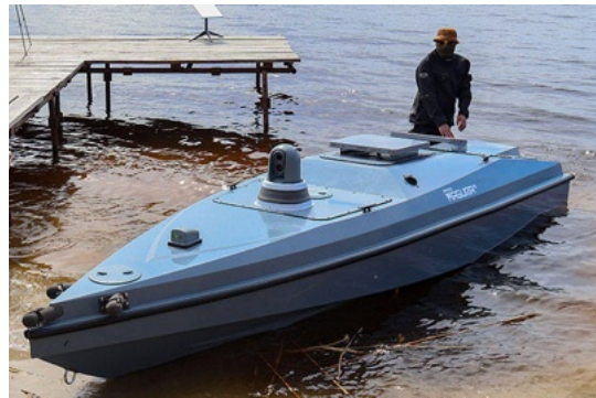
Figure 2: A MAGURA V5, a Ukrainian multi-purpose unmanned surface vehicle developed by the Ukrainian Defence Ministry (right).
