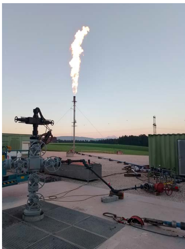
Testing of Zone 1 at the HOCH-1 shallow gas discovery well in Upper Austria. HOCH-1 is the first of three shallow gas wells planned for 2026
