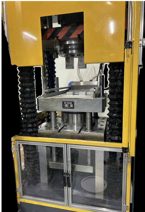
Figure 24. Semi-Automatic Hydraulic Press for Pucks Manufacturing. (Source: AEM)
