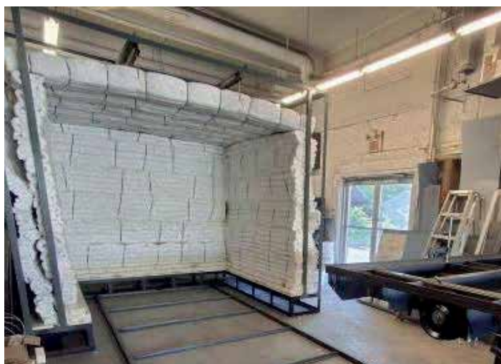
Figure 20. Inside of New Car-Bottoms Kiln (F04). (Source AEM)
