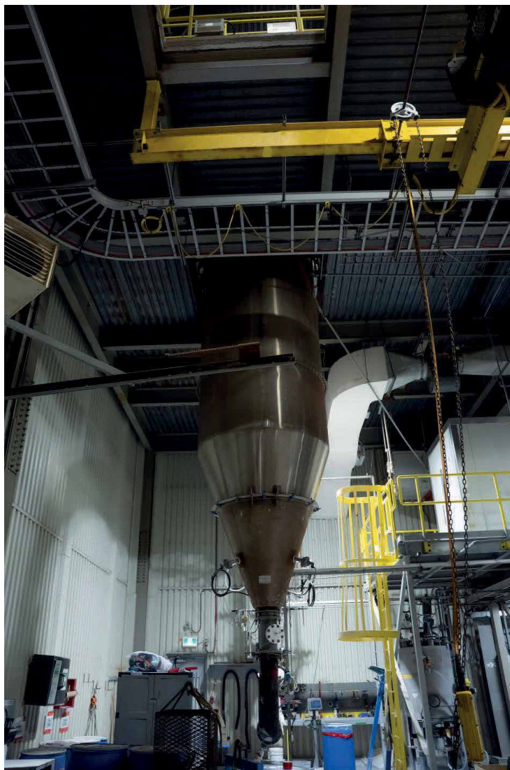
Figure 22. Bottom of Spray Dryer. (Source: AEM)
