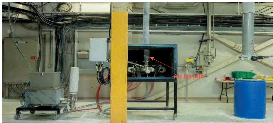
Figure 21. Air Jet Mill. (Source: AEM)
