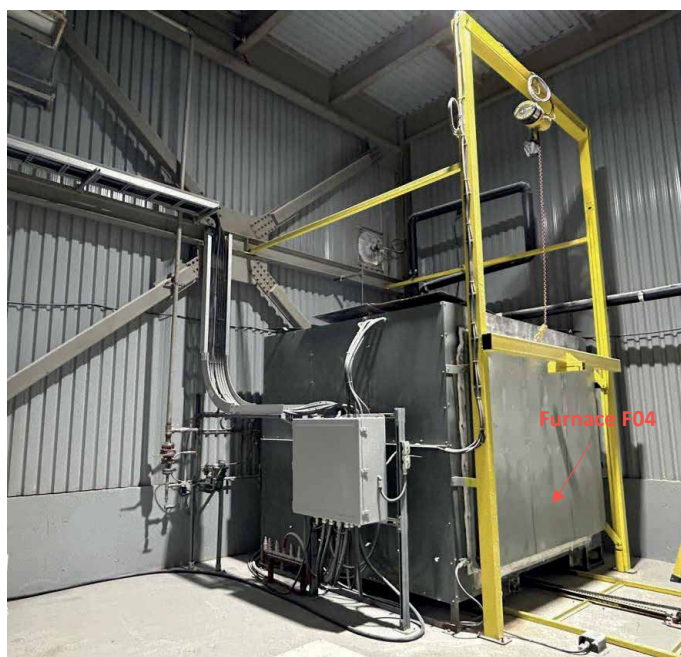
Figure 19. Outside of New Car-Bottom Kiln (F04). (Source: AEM)
