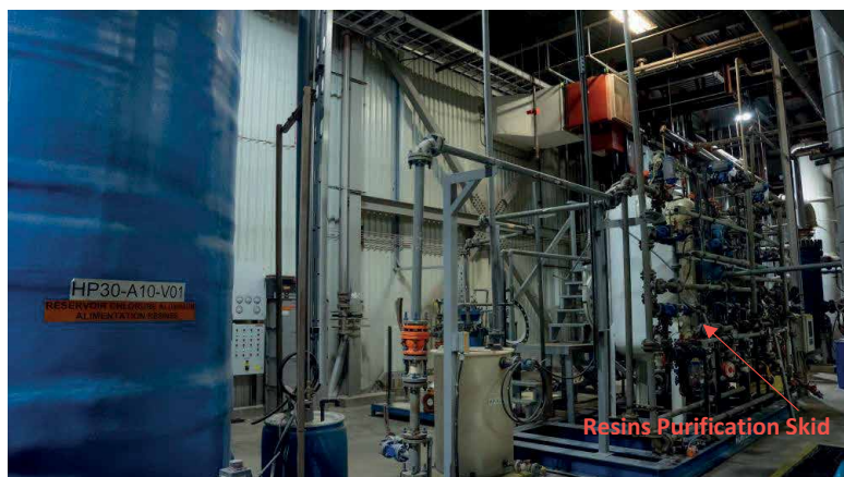
Figure 13. Resins Purification Circuit. (Source: AEM)
