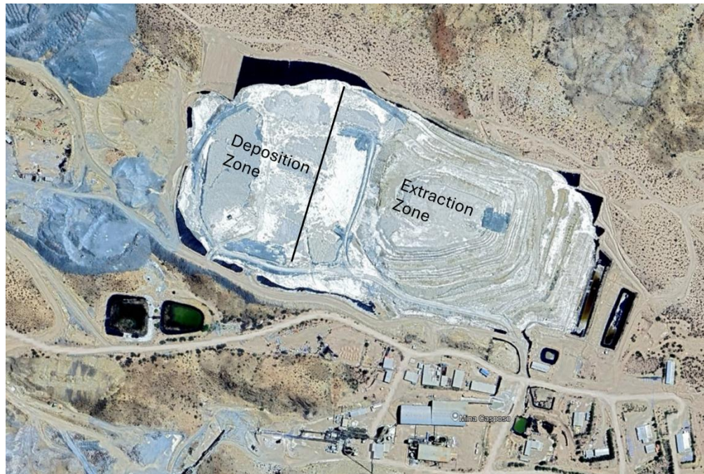
Figure 16.5: Extraction and Deposition zones - DCS
