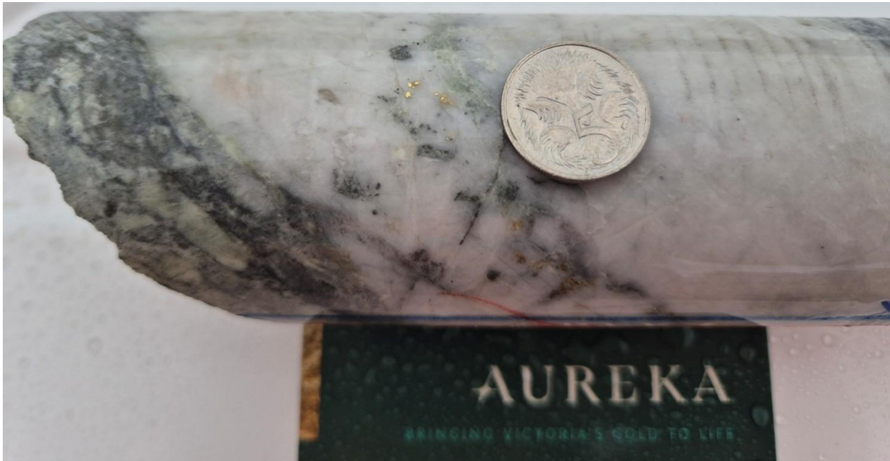
Figure 3. Drill core containing visible gold from RD048 at 413m: 10m @ 12.1g/t Au from 413m (inc. 0.3m @ 183g/t Au from 413m). 21
