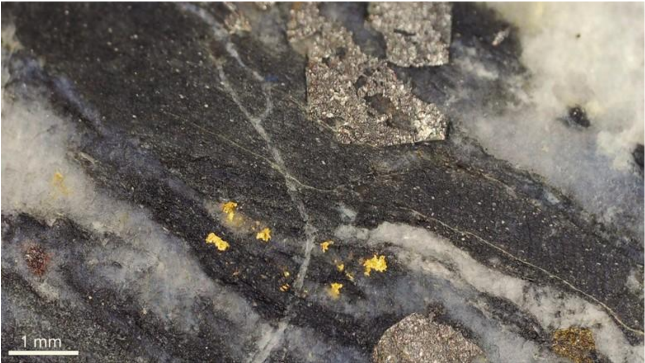
Figure 4. Microscope image of core from 25NED007 containing visible gold and pyrite at Comstock (St Arnaud) 14
