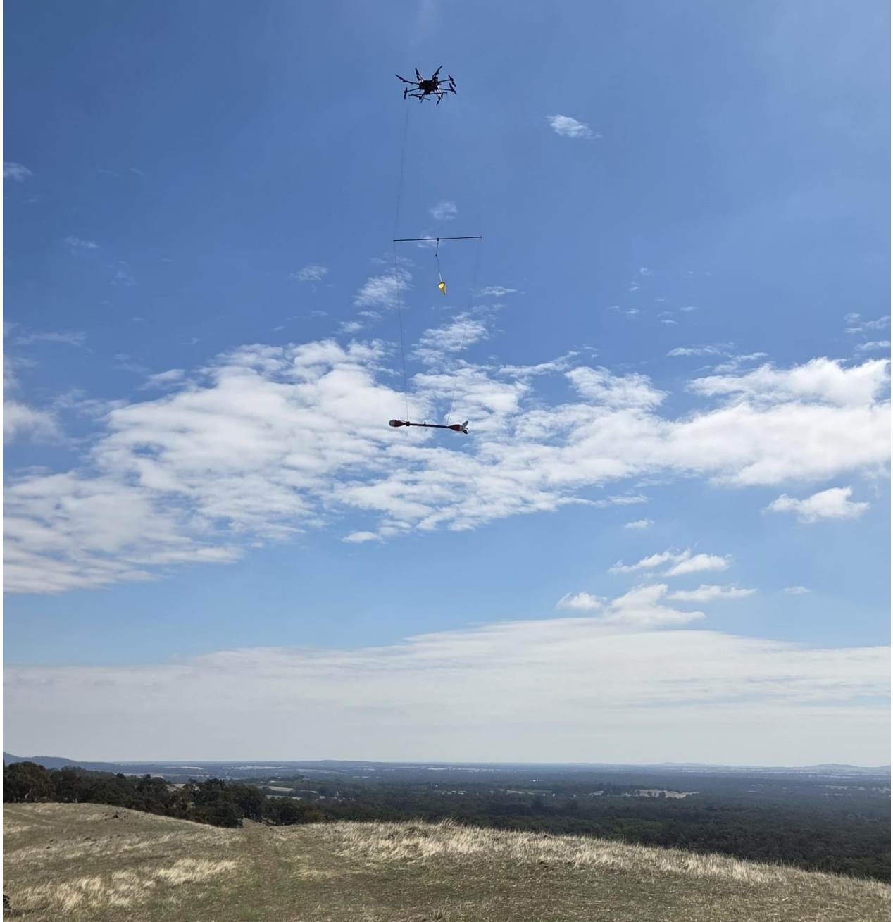
Figure 6: Airborne magnetic geophysical survey underway. Drone and connected magnetometer actively collecting data as it flies over the vicinity of Aureka's Irvine Project.
