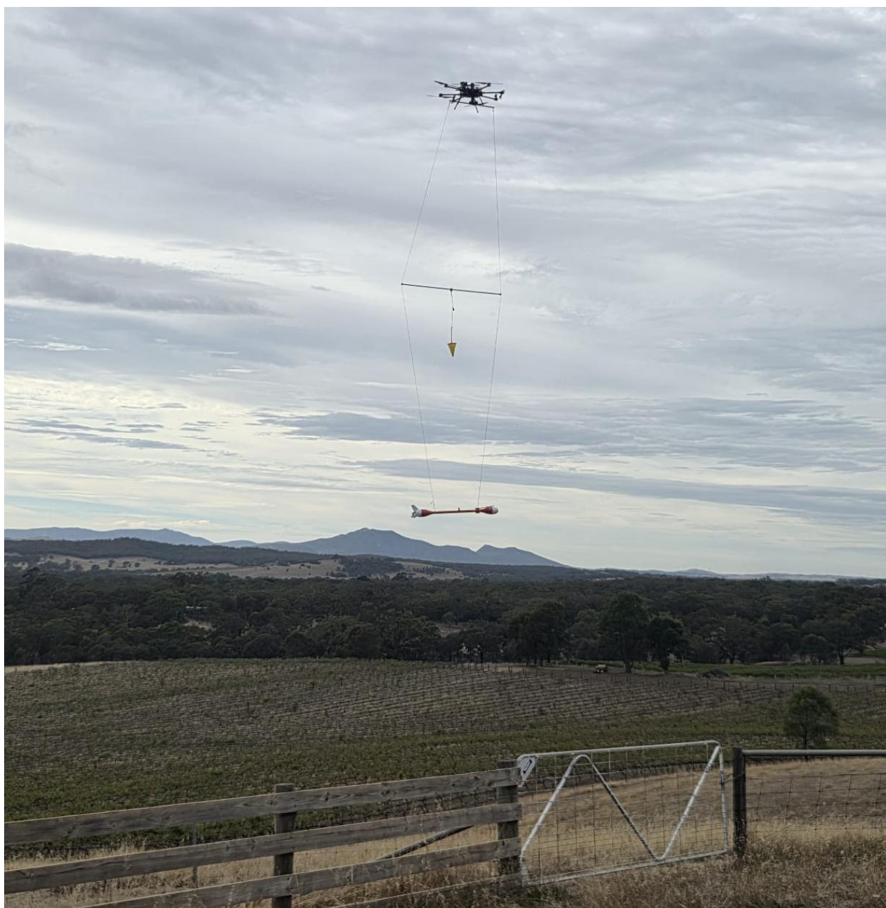
Figure 5: Irvine Project: - Drone and magnetometer actively acquiring data across the Irvine Project
