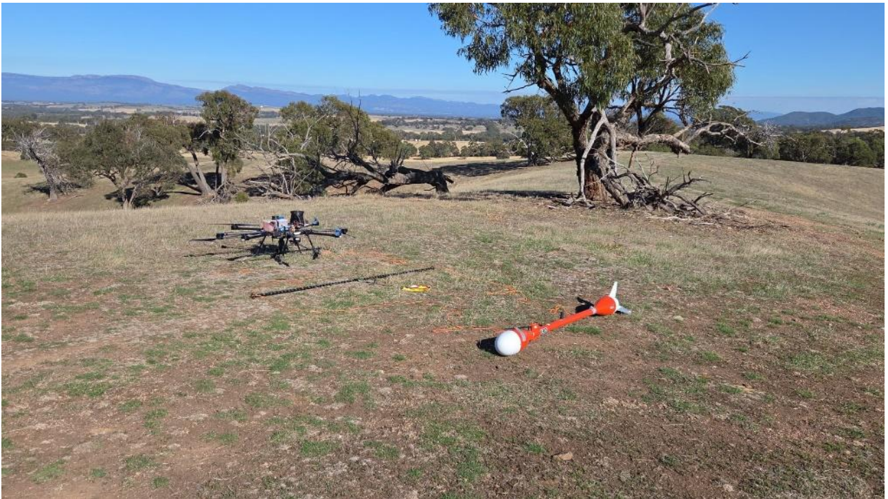
Figure 4: Irvine Project - Preparation of drone and magnetometer on the ground prior to commencement of survey
