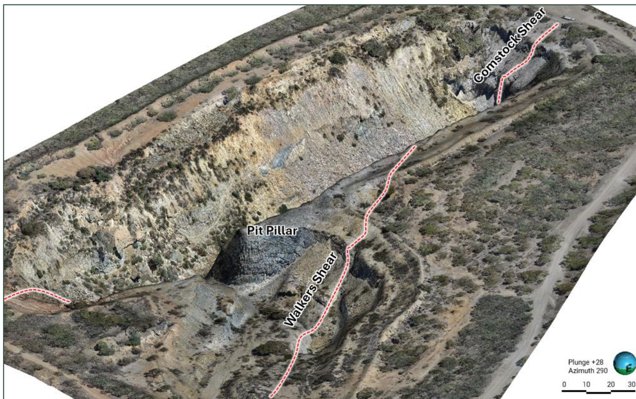
Figure 10: Comstock – View of the high-accuracy LiDAR and photogrammetry of the Comstock open-cut pit with key projected structures including the pit pillar – looking towards azimuth 290 27
