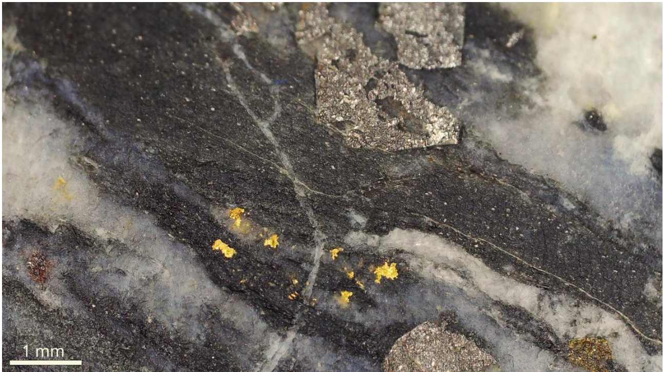
Figure 7: Comstock Project - Microscope image of core containing visible gold and pyrite 25NED007 23
