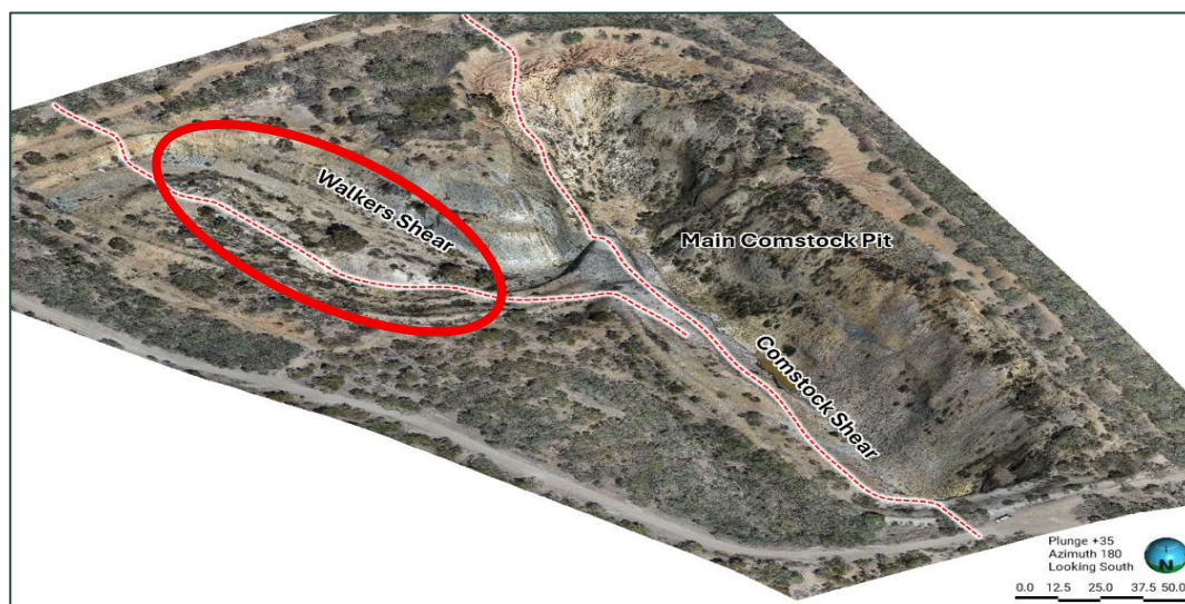
Figure 8 – View of the high-accuracy LiDAR and photogrammetry of the Comstock open-cut pit – looking towards the South (azimuth 18). Red circle highlights drill target area for the 6-week infill diamond drilling program now underway.
