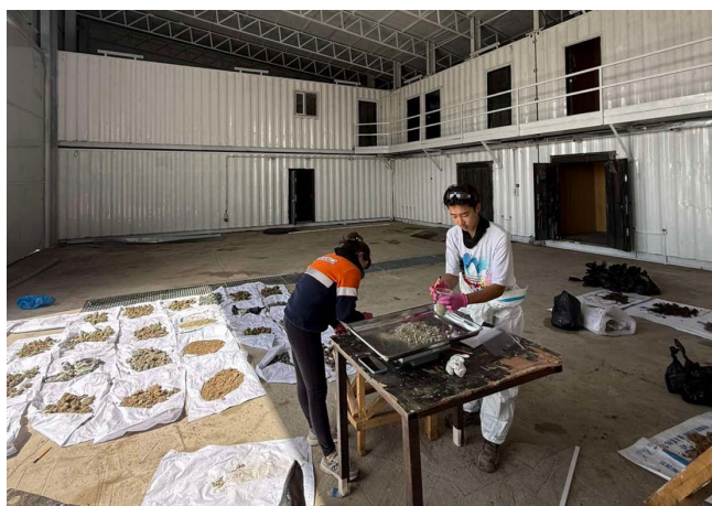
Figure 1. Preparation of geotechnical samples in the onsite workshop and warehouse.
