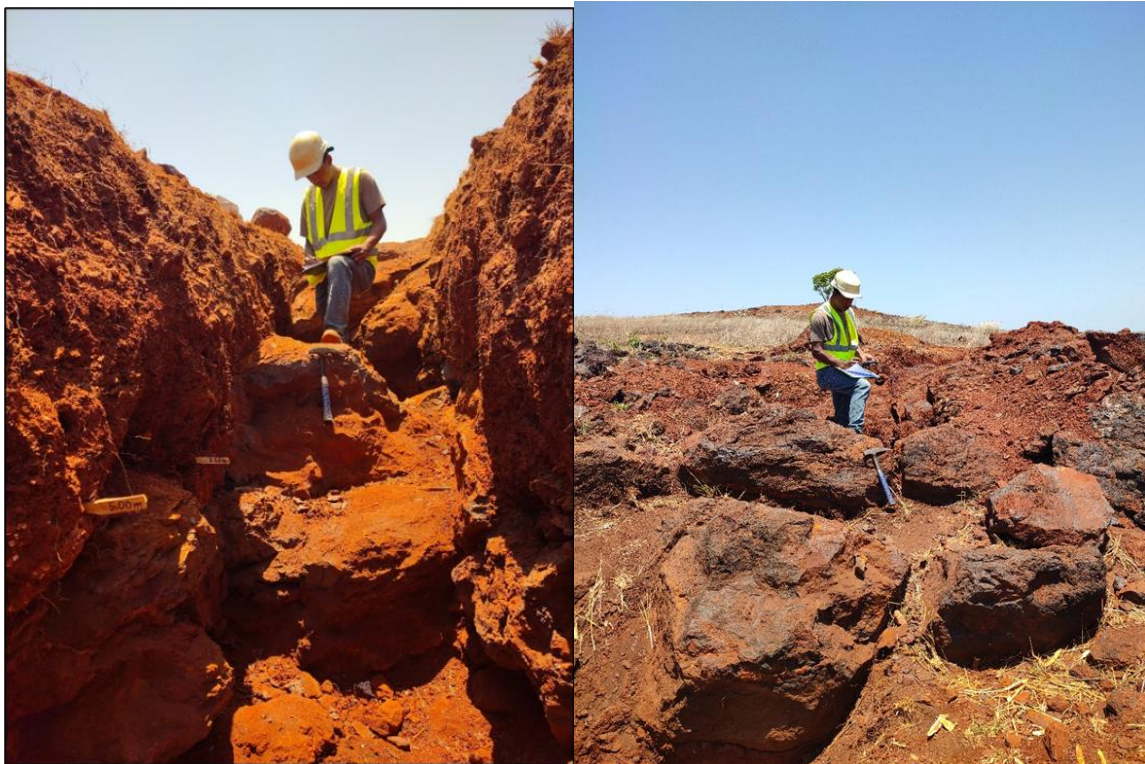
Figure 3 a) Massive Magnetite/Hematite at Trench BEKT006 (4.5 to 11.5m) b) Massive Magnetite/Hematite at Trench BEKT007 (6.0 to 18.5m)
