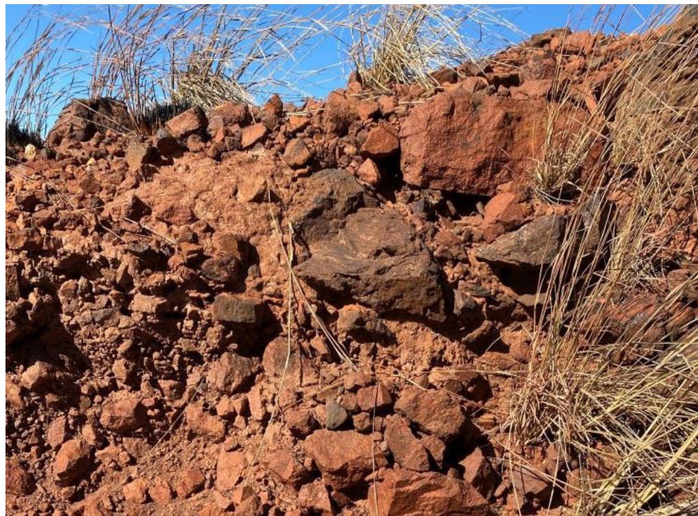
Trench 36: High-grade lump and fines iron ore DSO weathered zone, 2.2m at ~66% Fe*
