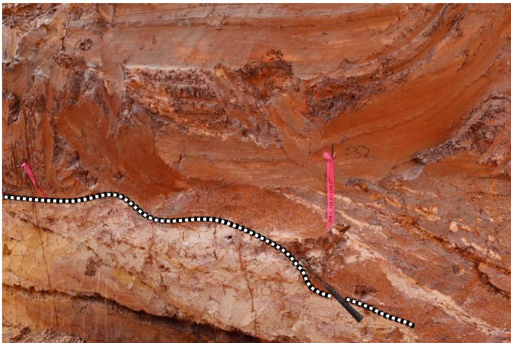
Figure 7: Trench 6A at 132m showing the sharp intermediate intrusive contact and alteration halo of phenocrysts.
