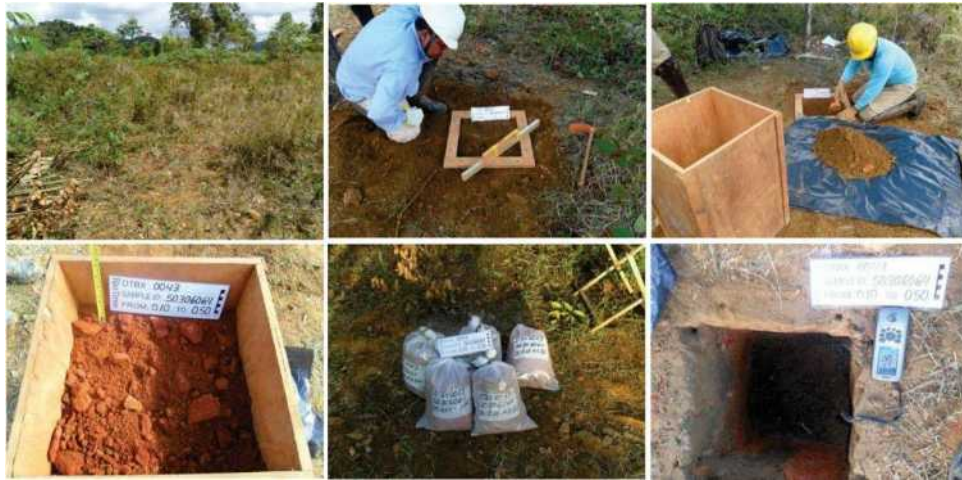
Figure 5-7: Bulk density measurements in situ pits
