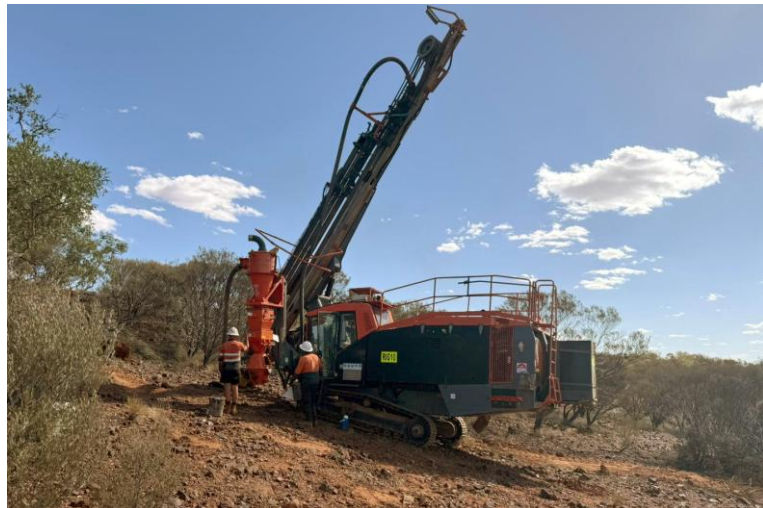
Figure 1: Castle drilling RC rig on site at Valley Bore
