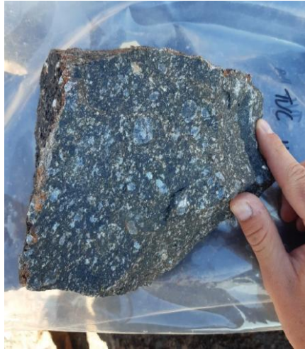
Figure 10 – Ultramafic-mafic rock taken from site 4, troctolite with the black minerals representing serpentinised olivine and the grey to white coloured minerals the two populations of plagioclase. The larger more rounded grey/white crystals are the plagioclase xenocrysts and the smaller subhedral to anhedral plagioclase believed to be primary intercumulus melt.
