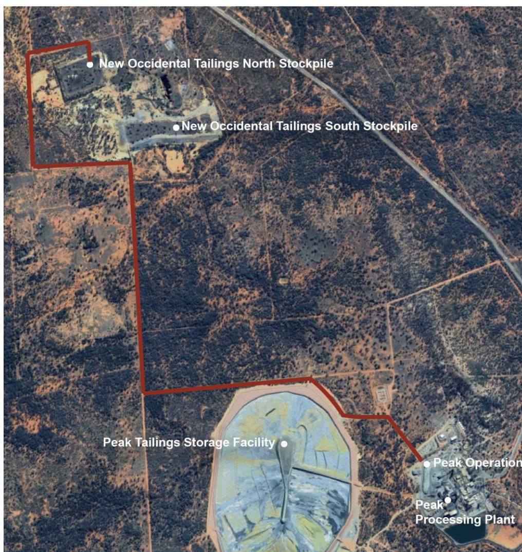
Figure 1: Satellite image showing the New Occidental tailings stockpiles and Peak processing plant, with haulage route (brown)
