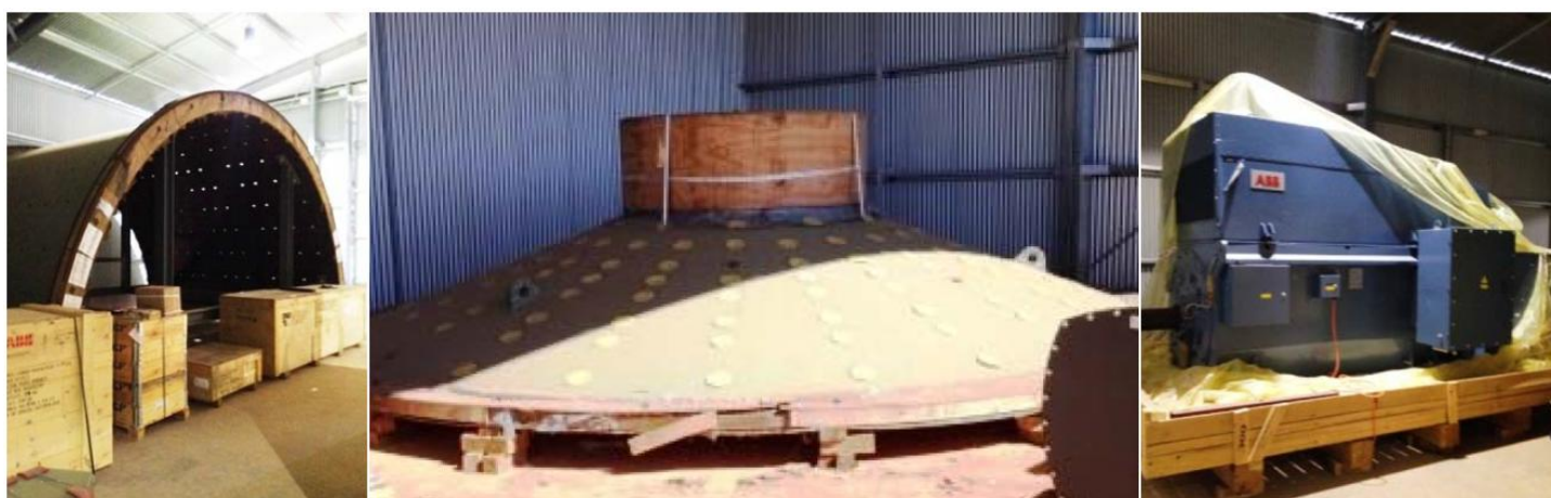
Figure 1. New SAG mill components and drive motors
