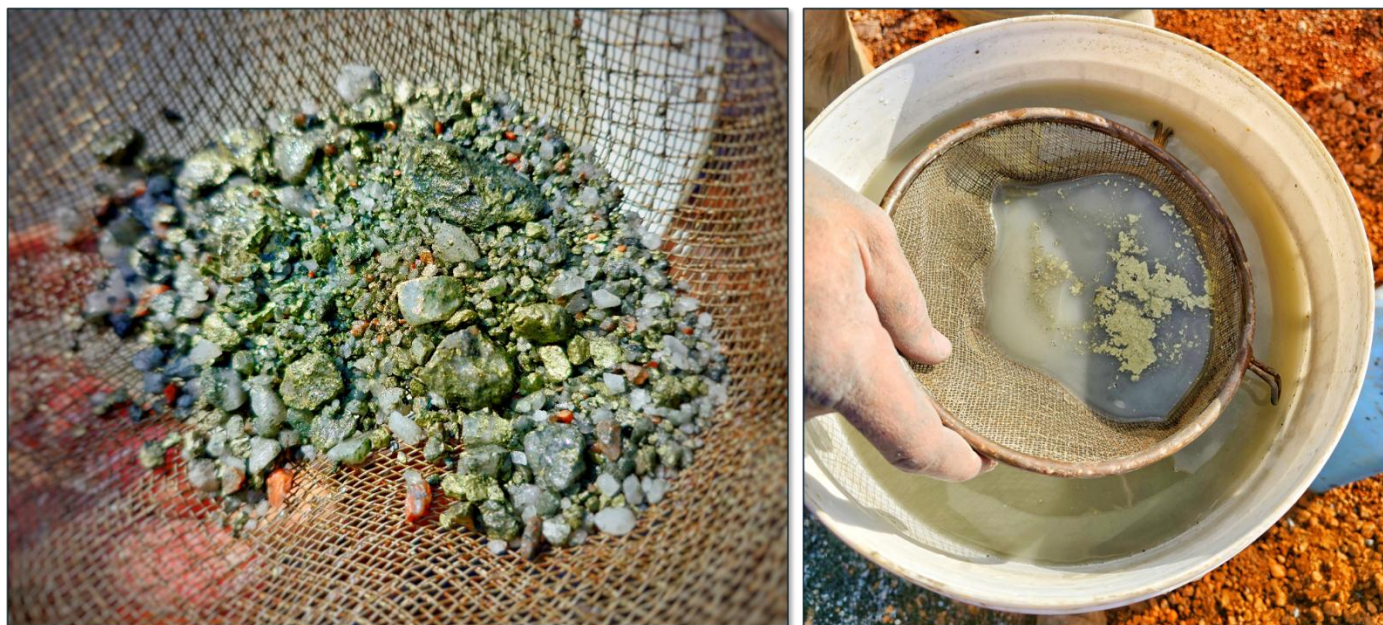
Figure 2: Semi-massive chalcopyrite-pyrite mineralisation intersected at 61m in 26SQRC006. This metre assayed at 8.98% Cu and 1.6 g/t Au (See Appendix 5)
