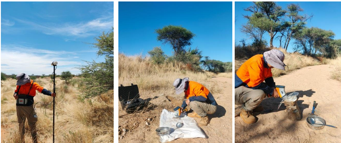
Figure 8: Site crew preparing magnetic survey preparations and soil and rock chip sampling.
