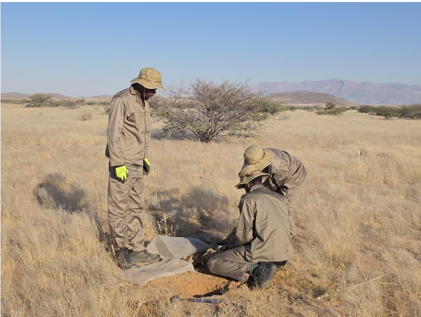
Image 1: Sampling team in the field at EPL 7626 collecting sieved soil samples.
