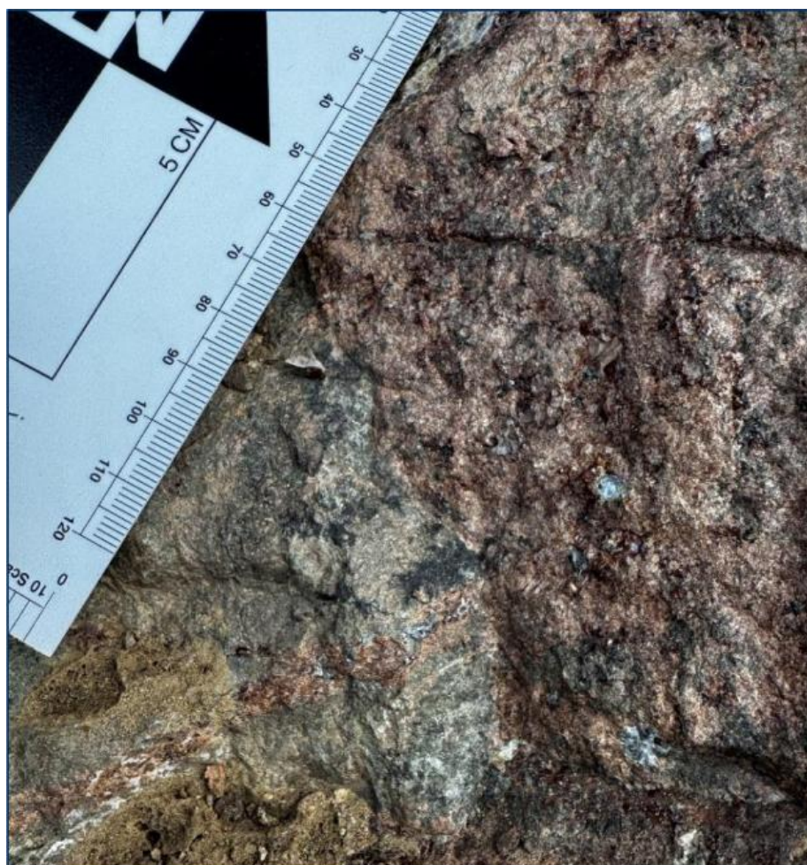
Figure 9: Rock chip sample 1939349 in Skarn contact zone, returned 2% (20,693 ppm) of Mo.
