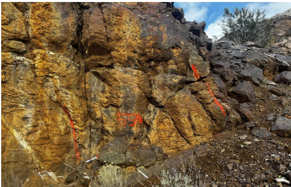
Figure 8: Channel sample ID 1080550 of limestone skarn that returned 4,191 ppm W from the northern section of the historic Garnet Mine, Alder Mining District, Elko County, Nevada. Five (5) holes are designed to test the immediate area.
