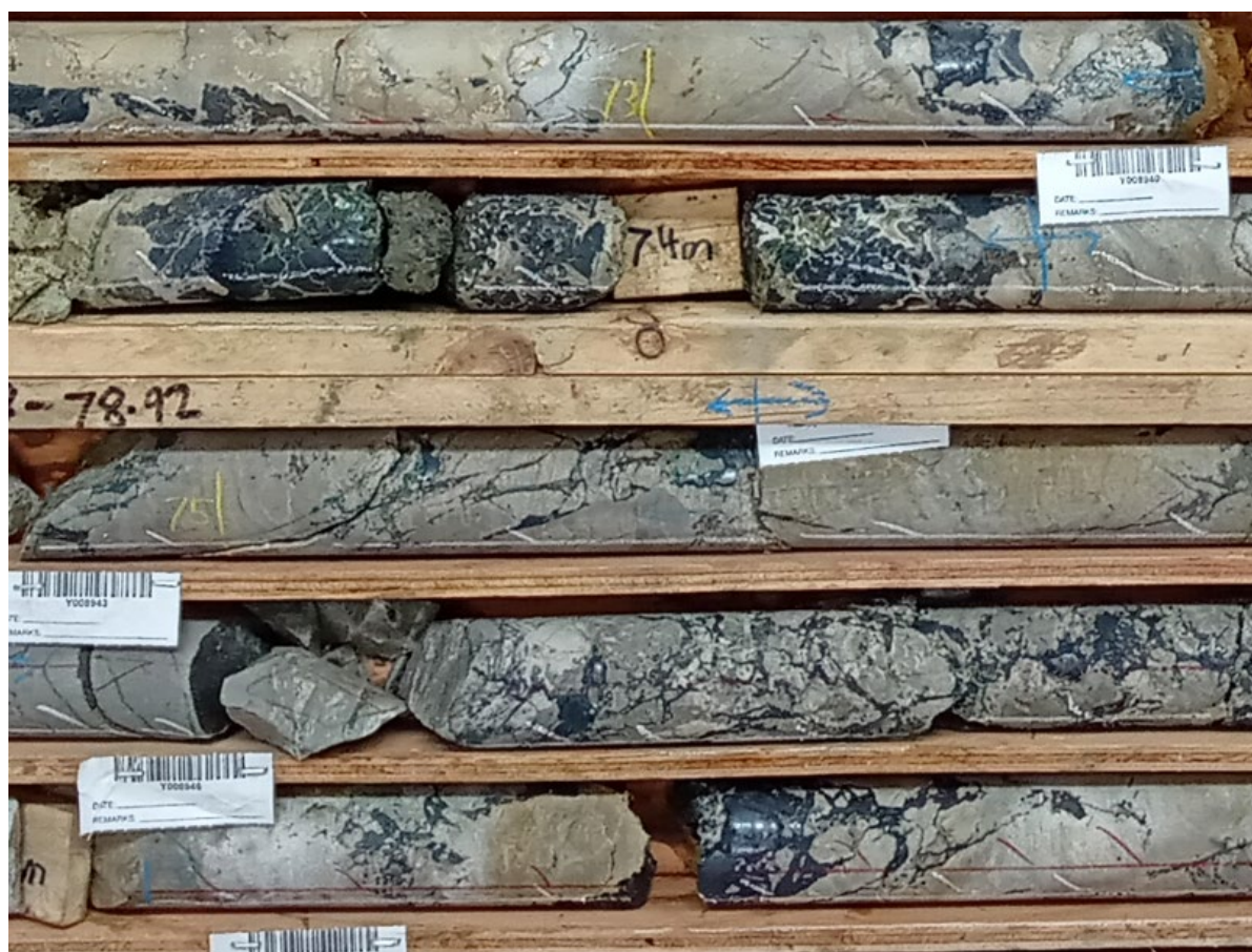
Figure 4: Dense semi-massive and breccia visual chalcocite (dark grey mineral) from PFS-002 (72.7-76.5m downhole). This interval assayed at an average grade of 8.1% Cu, 31g/t Ag.
