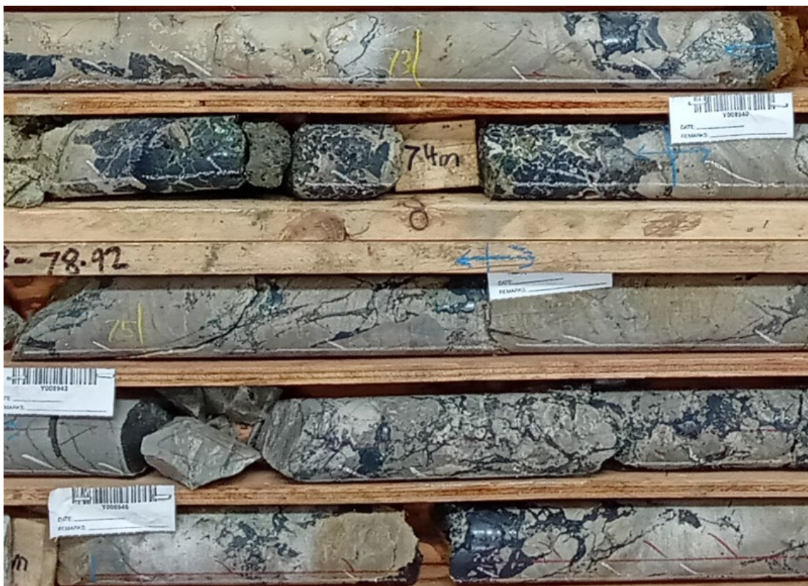
Figure 3: Dense semi-massive and breccia visual chalcocite (dark grey mineral) from PFS-002 (72.7-76.5m downhole). This interval assayed at an average grade of 8.1% Cu, 31g/t Ag.
