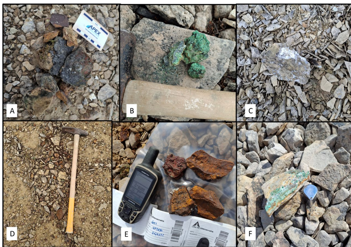
Figure 11: Examples of the interpreted copper gossans and outcrop from the Storm-Tornado area. For detailed descriptions of samples A-F above, see Table 3. Portable XRF was used to aid visual identification and these samples have not yet been analysed by laboratory.
