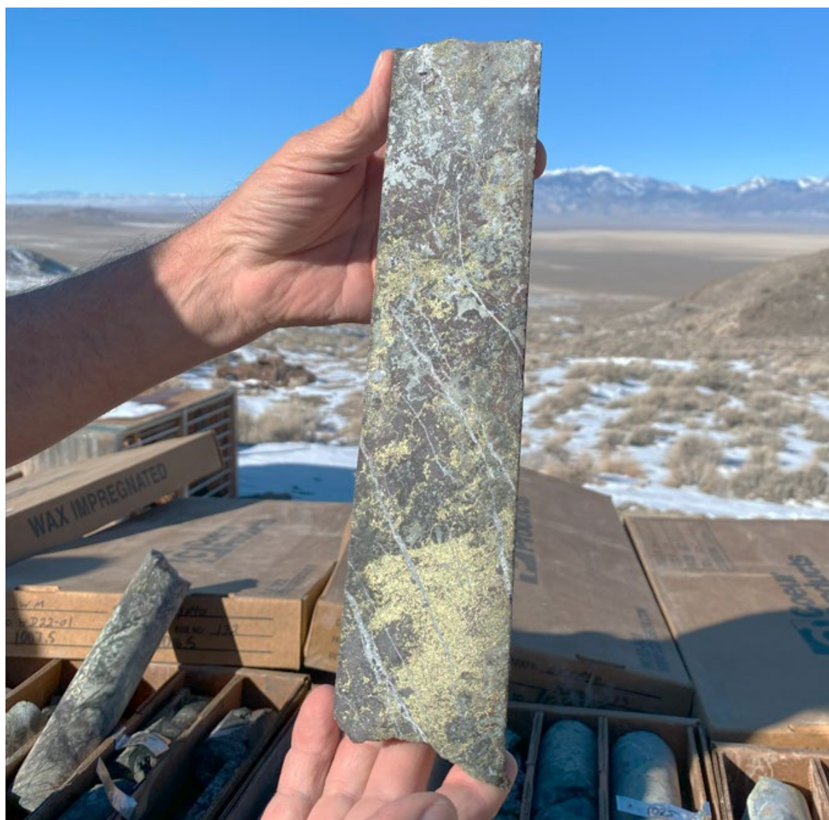
Figure 15: Cu-Au-Ag-In-Ga rich mineralisation in drill core from approximately 422m (1,385ft) downhole in WD22-01c (see Table 13 for interval details).
