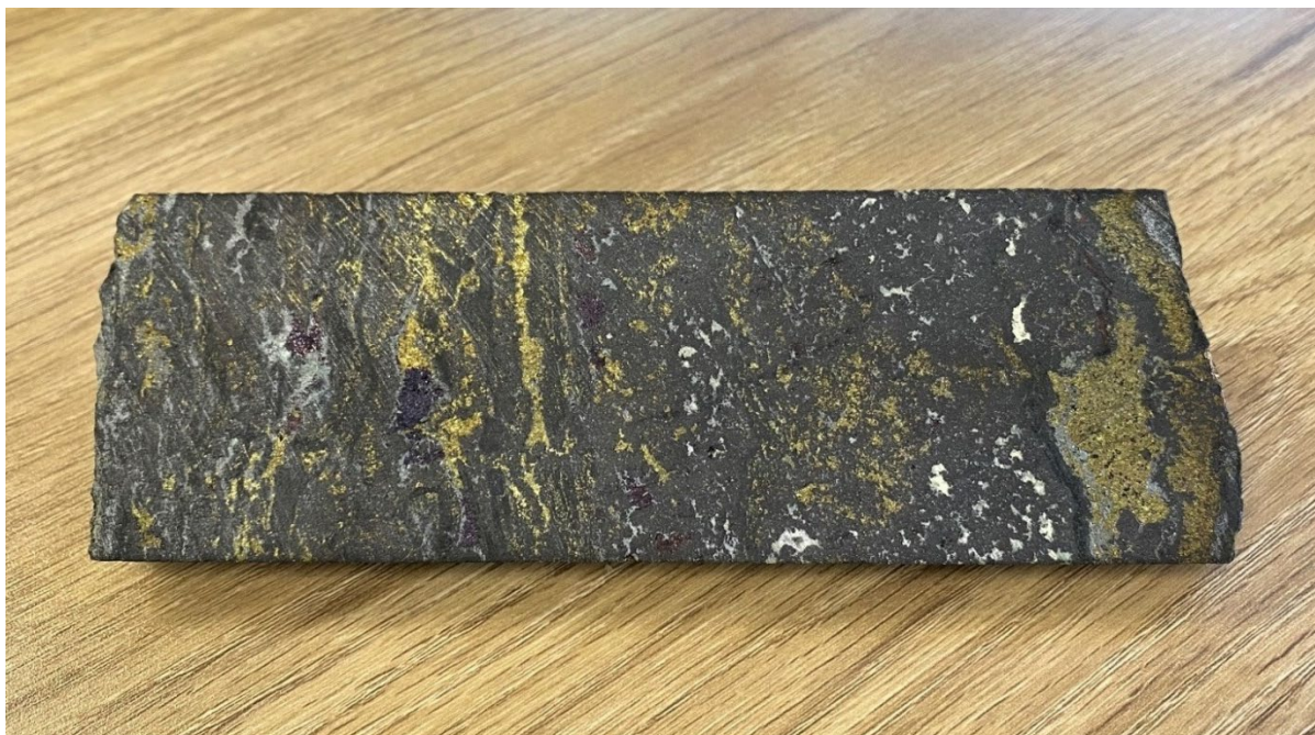
Figure 2: Drill core from previously released diamond drill hole WD22-01 from approximately 544m (1,785ft) downhole from the ‘Goldilocks Zone’ which assayed 95g/t In, 2.8% Cu, 0.5g/t Au, 39g/t Ag.
