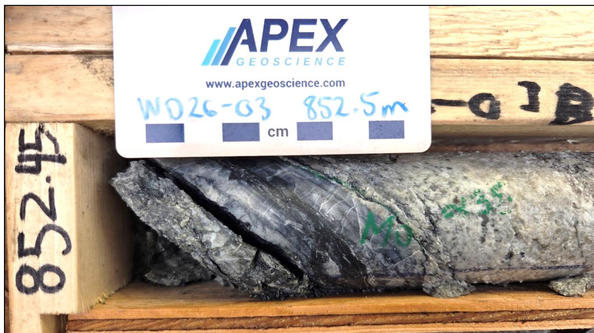
Figure 7: Very strong visual molybdenite (blueish-grey)-quartz-pyrite veining in NQ drill core from approximately 852.45m downhole in drill hole WD26-03. Laboratory assays for this interval are pending.
