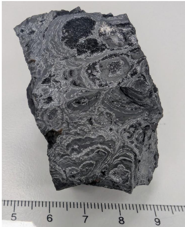
Figure 2: High-grade manganese rock chip sample from El Largo corridor grading 56.7% Mn 1 showing manganese oxides as pyrolusite and rhythmic banding related to hydrothermal deposition
