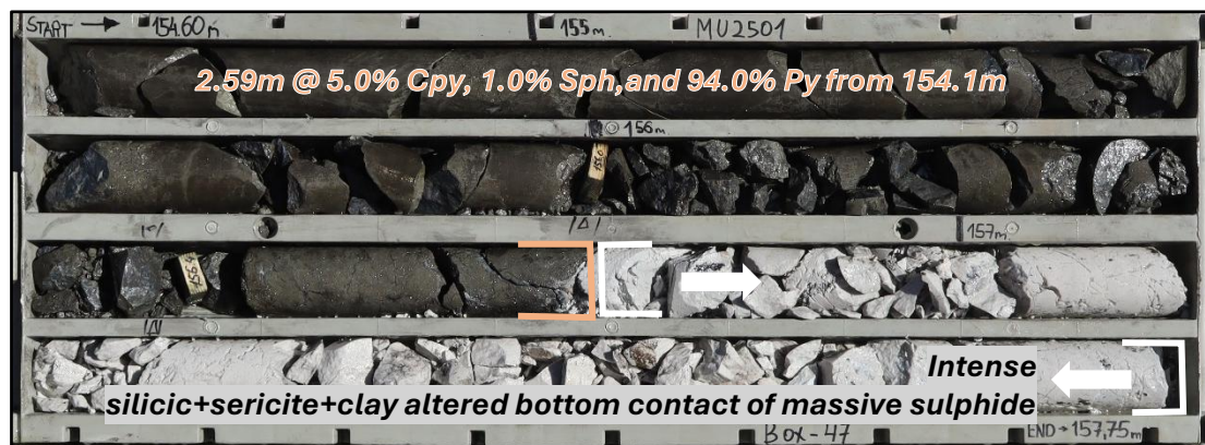
Photo 1: The massive sulphide mineralisation in drillhole MU2501. Mineral abbreviations are provided in Table 1.
