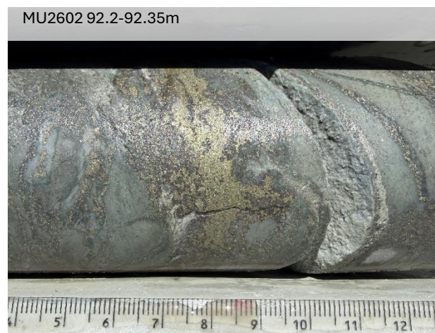
Photo 4. Oxidised rhyolite with azurite and malachite staining, drillhole MU2602.
