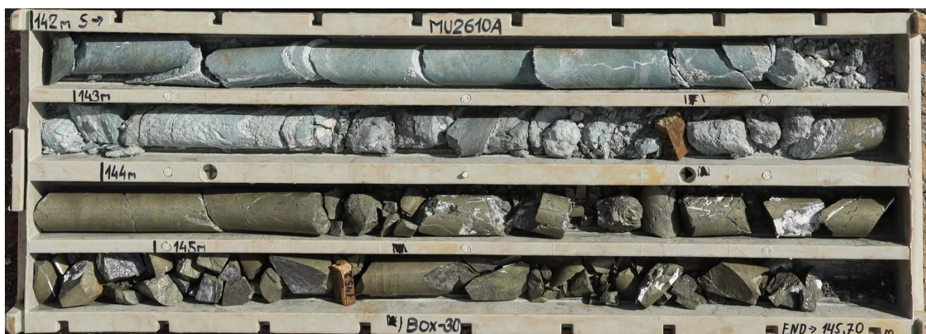
Photo 2. Chalcopyrite-rich massive sulphide mineralisation (from 143.85 m), drillhole MU2610A, box 30 (142.0 to 145.7 m). Visual estimates of mineral abundance are provided in Table 1.
