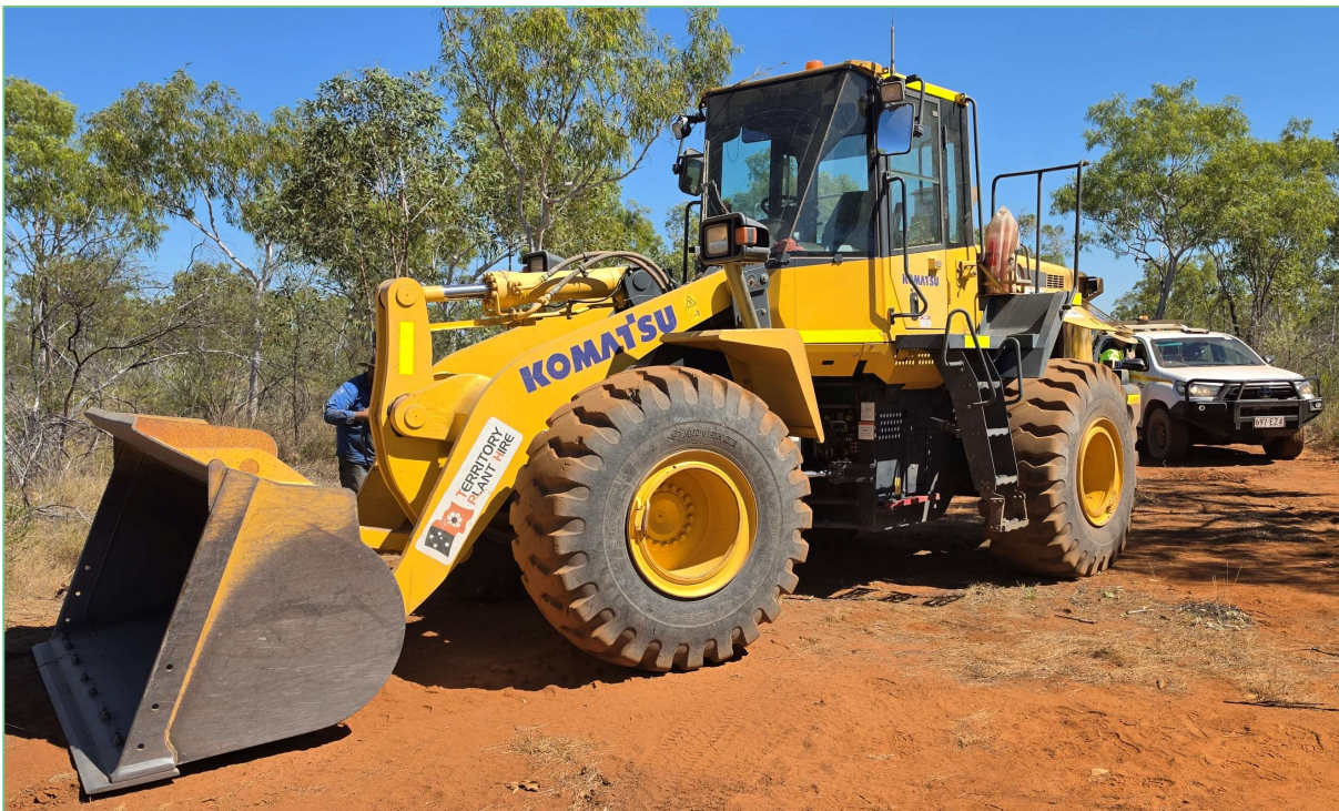
Figure 5: Front end loader used for preparation of drill pads and access tracks at the Barkly Project.
