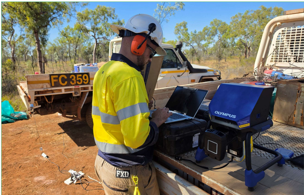
Figure 9: pXRF chemical analysis during drilling at the Barkly Project.
