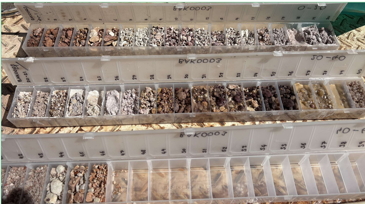
Figure 7: Stratigraphic profile logging of drill chips sampled from a 60-m deep drillhole at the Barkly Project.
