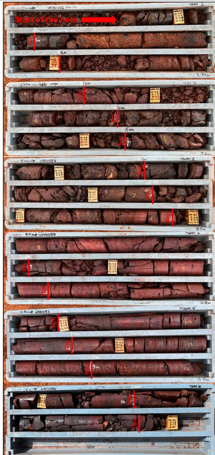
Figure 3. Drill hole WDDD056 twinning hole WDRC056 that intersected 13m @ 59.3% Fe & 0.7% Mn from 1m including 7m @ 62.0% Fe & 0.7% Mn from 7m. Assays quoted from the equivalent interval from WDRC056 to the twin diamond hole will vary due to geological variation and recovered core. High grade iron mineralisation can be observed from 8 to 14m depth. Downhole metre marks are drawn on the core and tray ribs.
