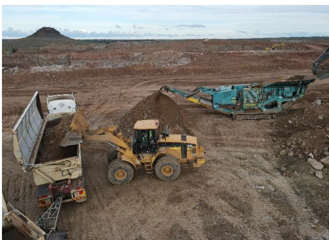
Figures 7 & 8 – Open Pit & ROM operations at the Pinnacles Mine with haul truck loading for transport to Rasp Mill
