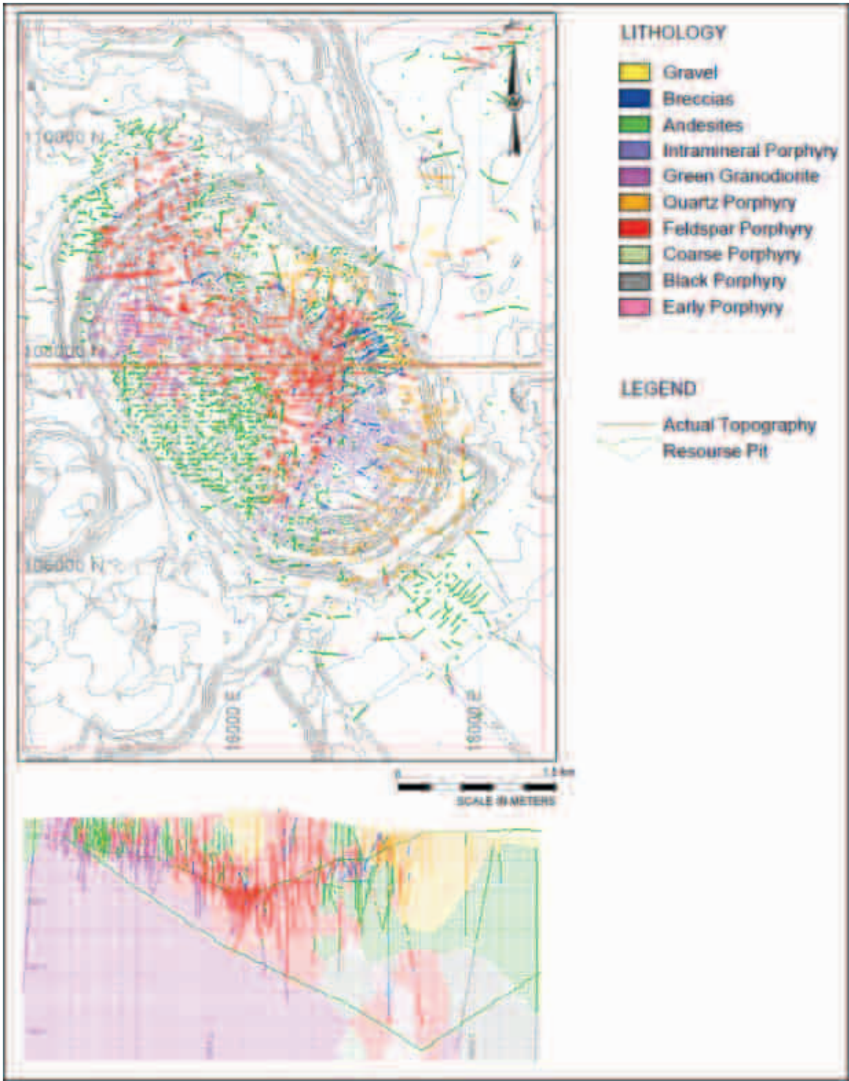
Figure 7-6: Lithology Model Plan View and Vertical Sections, Escondida
