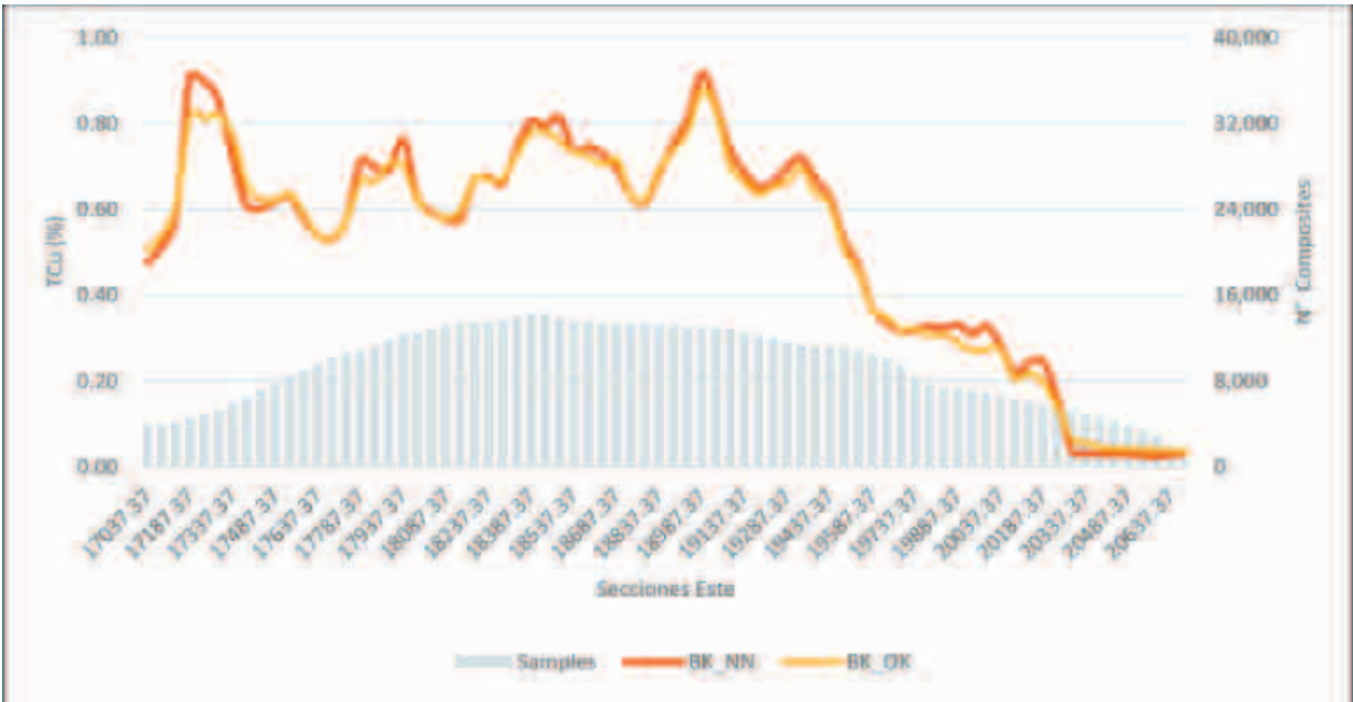
Figure 11-16: Swath Plots Total Sulphide, Escondida
