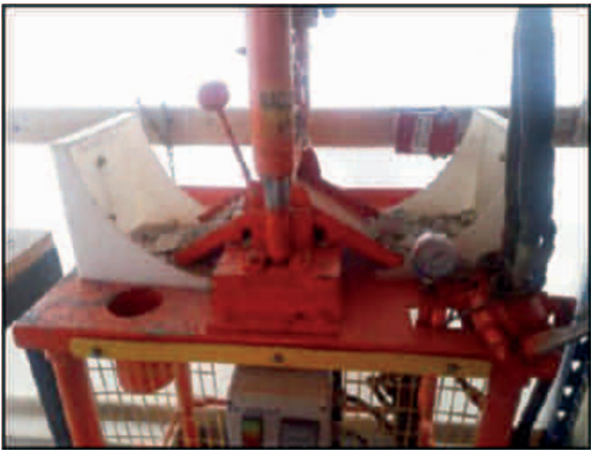
Figure 8-5: Hydraulic Guillotine for Core Cutting
