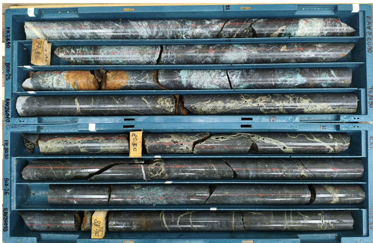
Figure 4. Semi-massive to massive sulphide breccia with matrix of sulphide (dark fine grained material) and vuggy silica alteration from 76m to 83.6m. Interval did not return significant precious or base metal mineralisation but is indicative of a large-scale epithermal system
