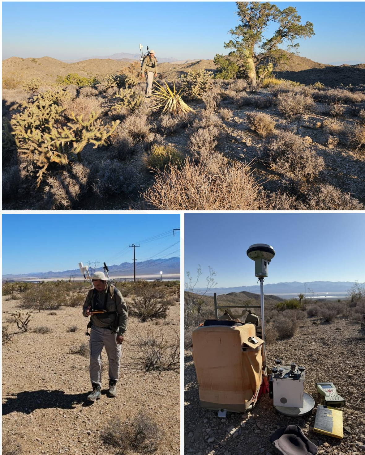
Figure 1: Field crew conducting ground magnetic and gravity survey at Desert Star Project
