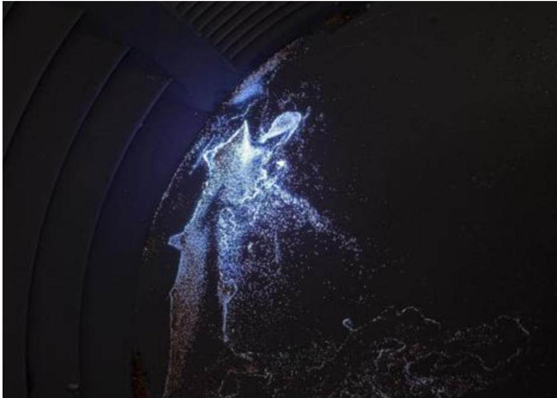
Figure 5 UV fluorescent scheelite observed within a hand-panned concentrate from 25GLR070 505-506m. Original RC sample (unconcentrated) returned assay 0.94% \text{WO}_3 . The image demonstrates the coarse-grained nature of scheelite mineralisation observed within the Glenburgh Gold System.
