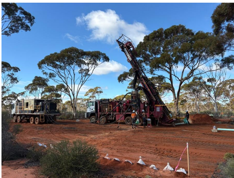
Figure 1 - RC Drilling underway at Beachcomber
