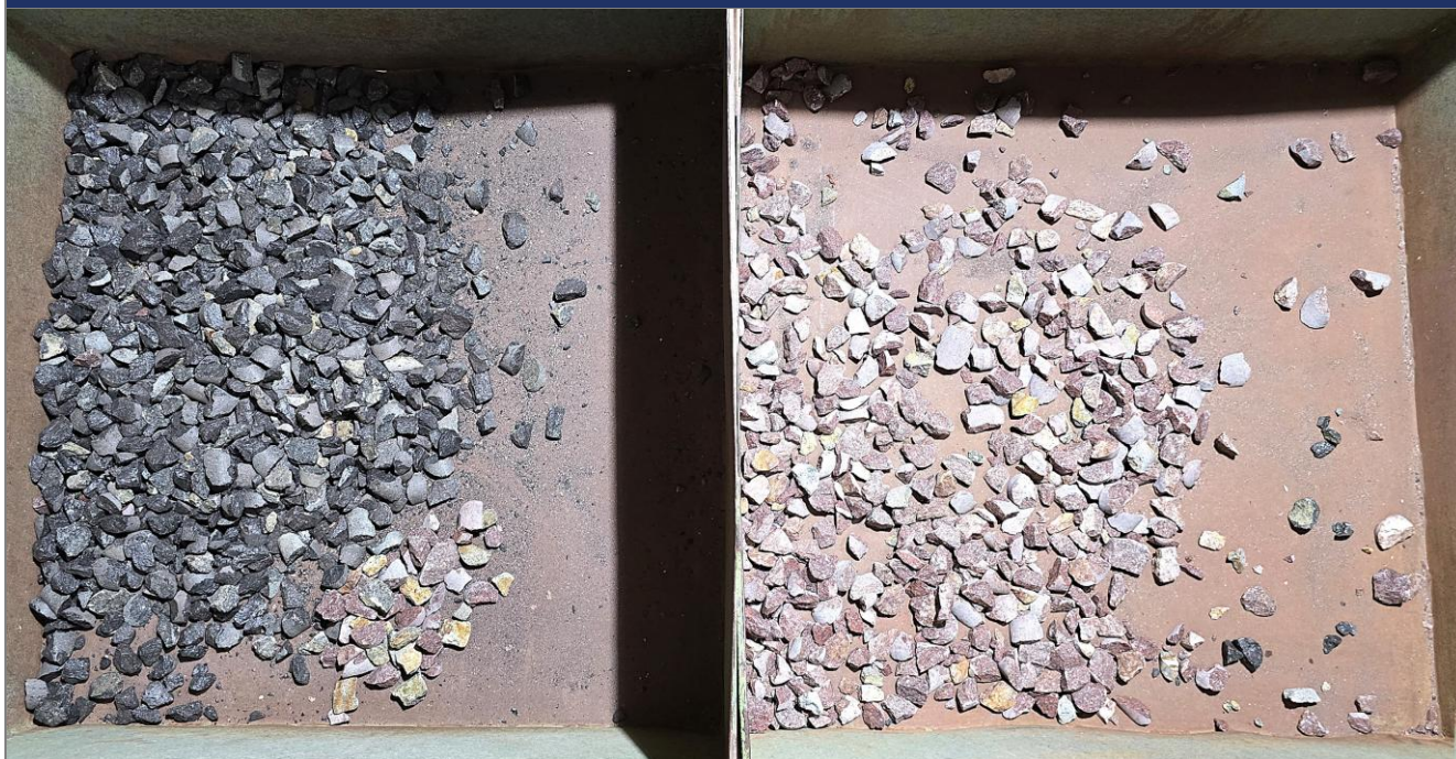
Drop (left) and Eject (right) sorter fragments showing clear separation of dark ultra-high grade Monte Alto mineralisation
