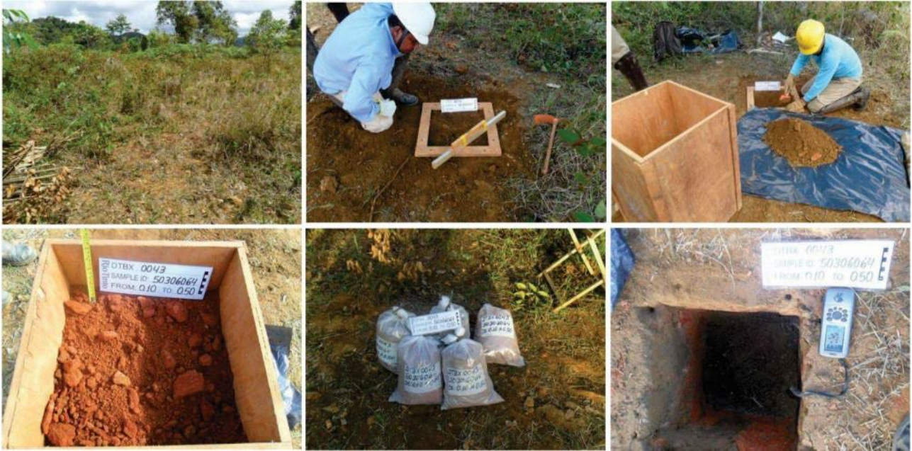
Figure 5-7: Bulk density measurements in situ pits
