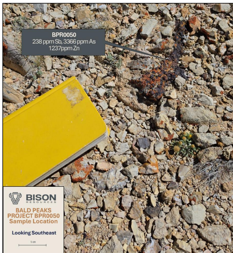
Figure 4: Rock chip sample BPR0050 (660,441mE, 4,460,263mN, 2,373mRL) in-situ subcrop showing iron oxides in carbonate at the Bald Peaks Project 5 .
