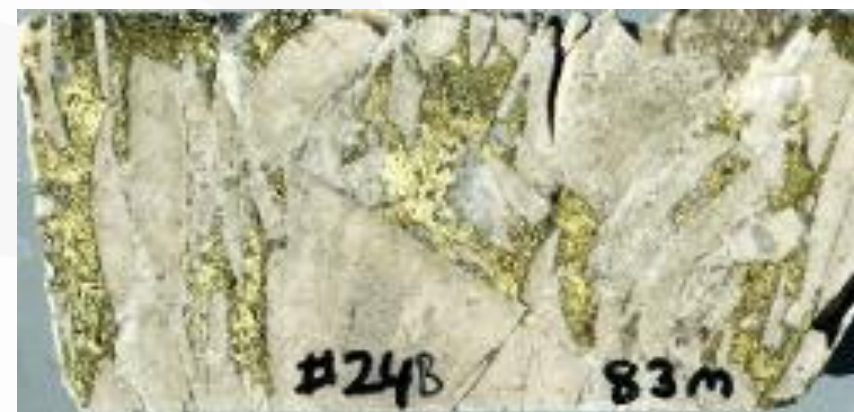
24CAEDD024B 83.1m. Interval 82m to 84m 3.04% Cu, 0.23gt Au, 102.9gt Ag
