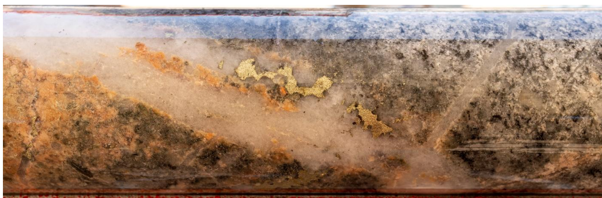
Figure 4 Composite B-vein with quartz and chalcopyrite in altered granodiorite porphyry at 525.5m downhole depth in 25BRD0037. From within a 17.4m wide interval visually estimated to contain 0.75% chalcopyrite (0.25% Cu*). Core diameter 61mm.
