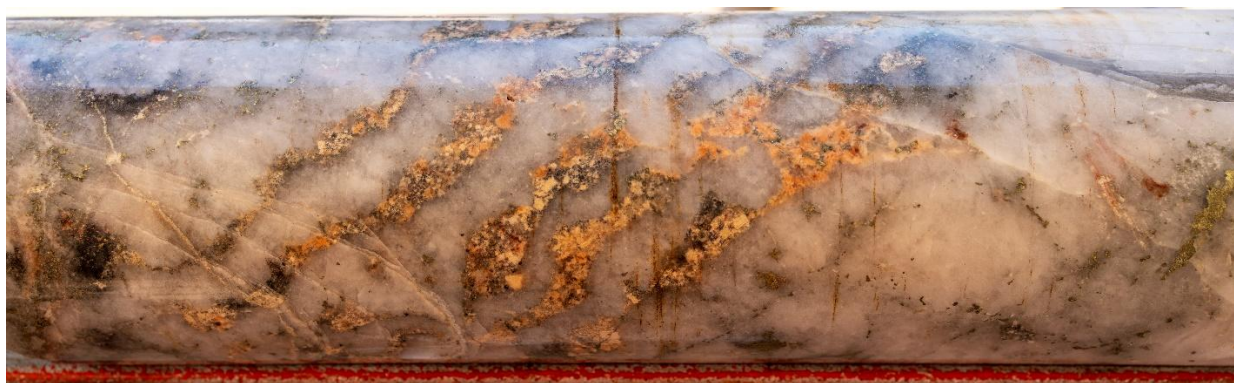
Figure 5 UST textured magmatic quartz body at 495.7m downhole depth 25BRD0037. From within a 0.6m wide interval visually estimated to contain 1% chalcopyrite (0.35% Cu*). Core diameter 61mm.
