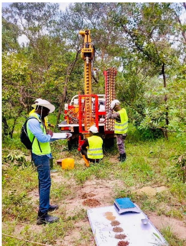
Figure 3: The Castle team advancing auger drilling operations on-site and collecting key samples.
