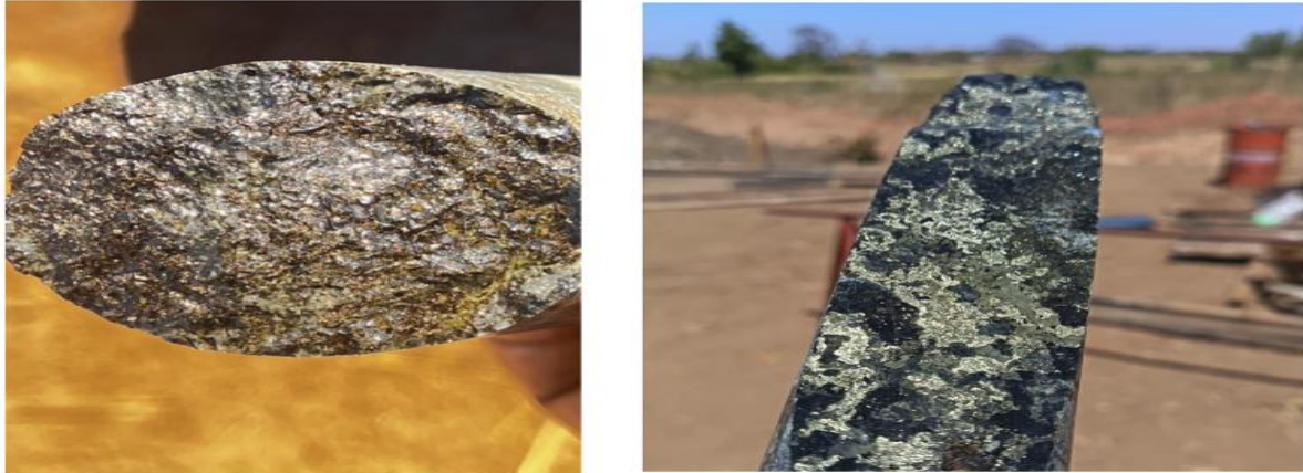
Figure 6: Breccia and sulphide alteration in diamond drill core from the Chilwa carbonatite system : MPYDD001: Sulphide alteration in NQ core at a depth of 85m downhole. For full results pertaining to MPYDD001 refer ASX Release dated 20 October 2025 (“Elevated REE Grades Confirm Carbonatite Discovery”)
