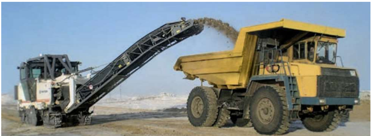
Fig 1 – Surface Miner direct loading
