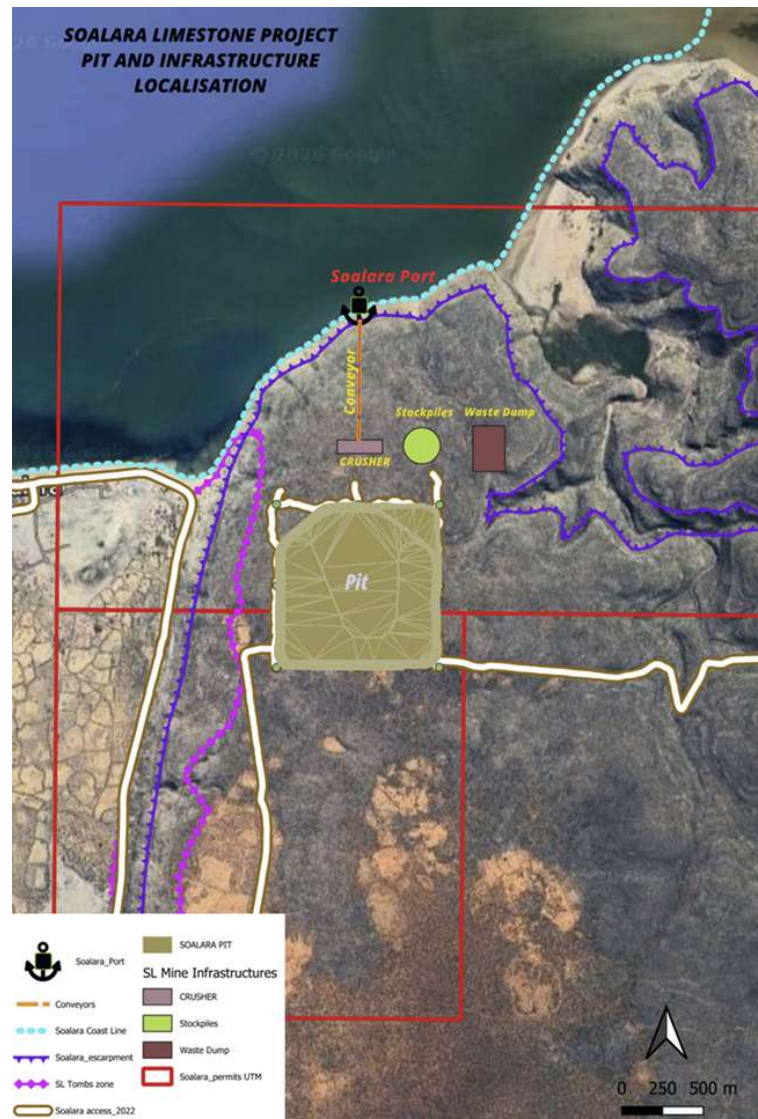
Fig 4 – Preliminary Mine Site Layout
