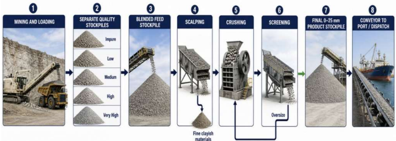
Fig 3 – Limestone Processing Flowsheet (nominal sub-25mm shown)
