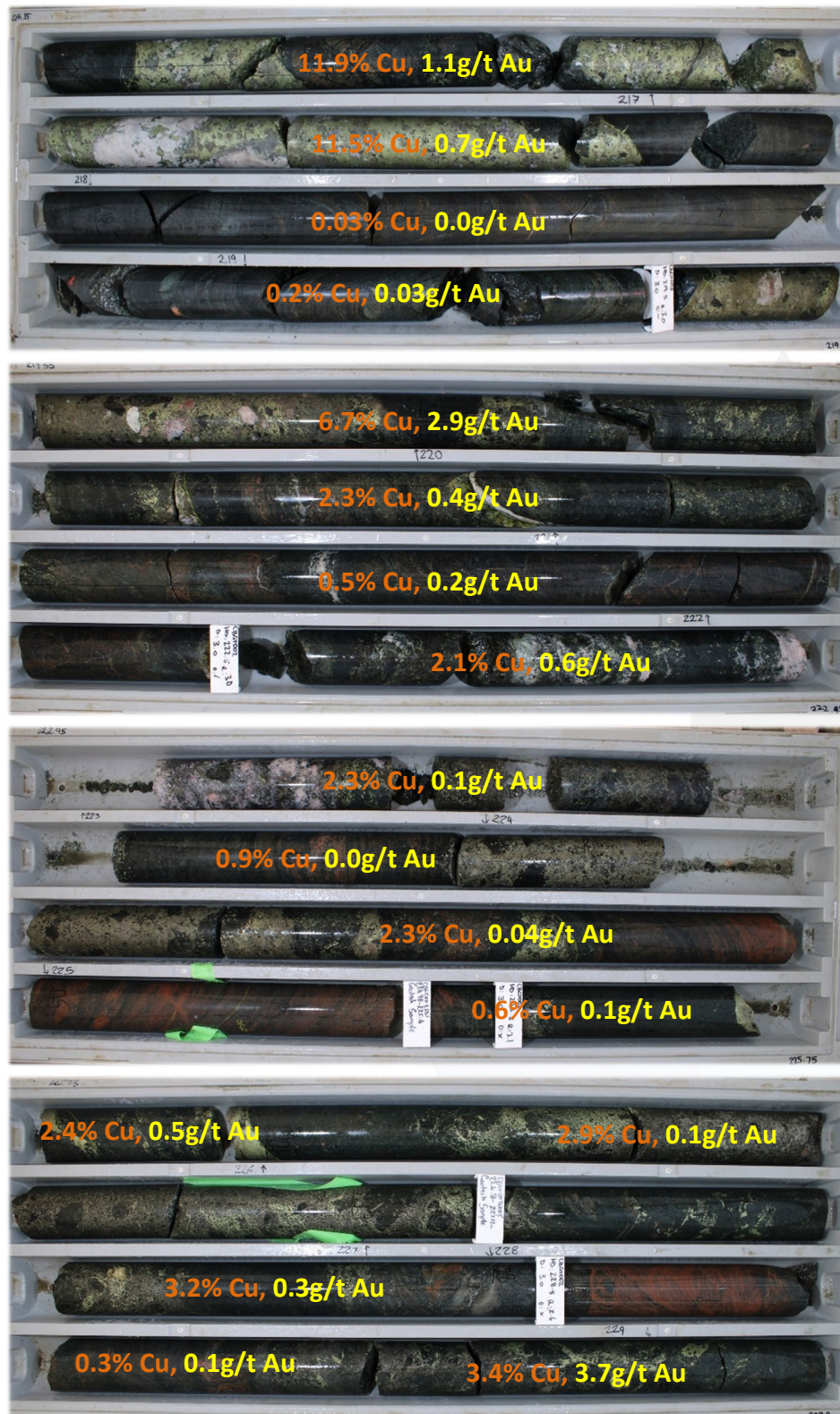
Image 1. CBGT002 core photos showing high grade mineralised intercept averaging 13m (TW~12m) @ 4.0% CuEq from 216m to 229m.
