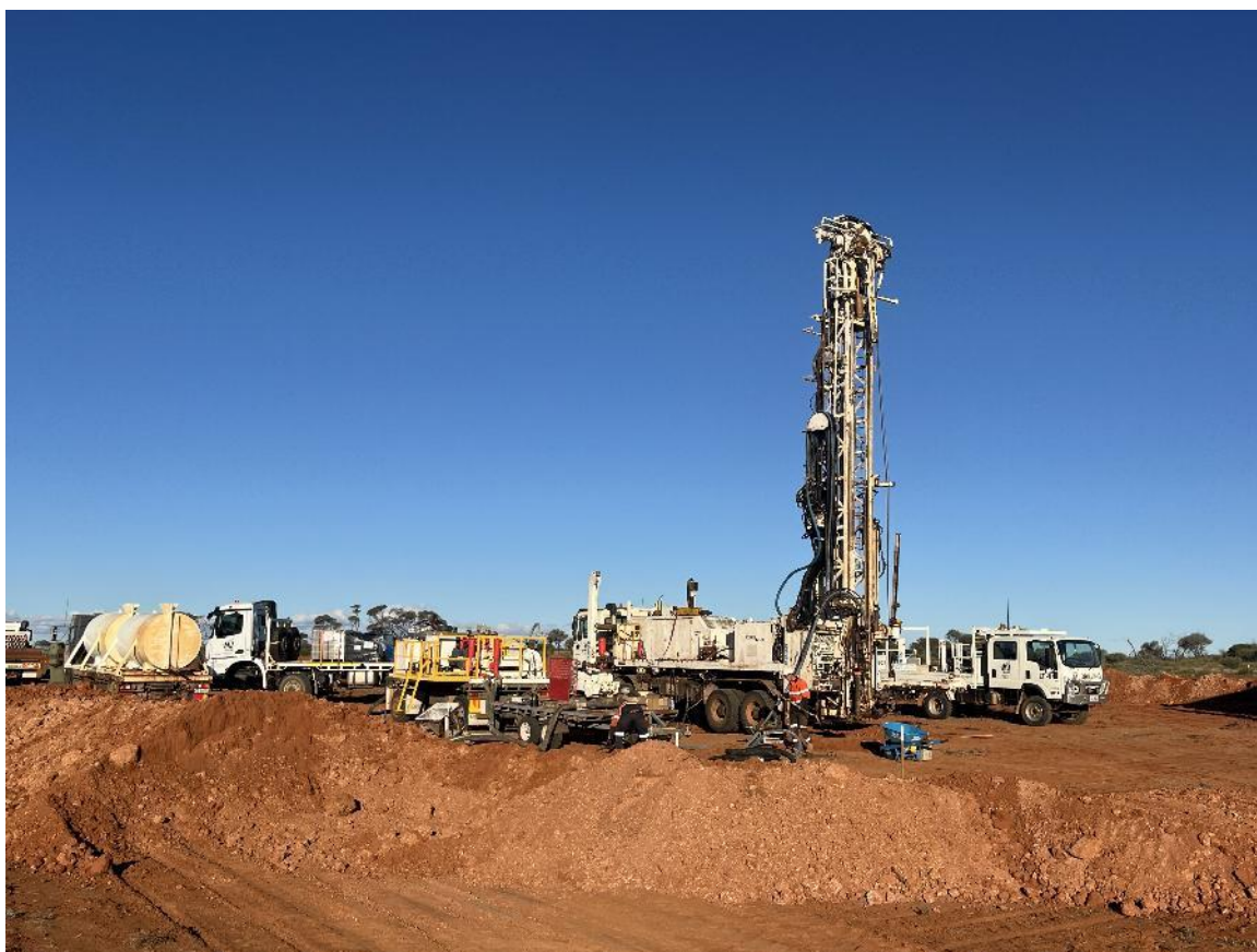
Figure 1: Hydrogeological drilling ongoing at Windabout subsequent to quarter end.
