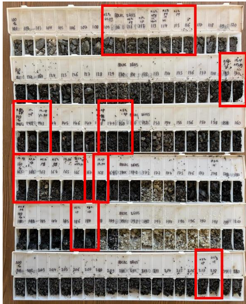
Representative RC rock chip samples from drill hole BDCRC26015 (101–250m EOH), with intersection Pyrite (~0.1–0.2%) observed from 109–116m, Chalcopyrite (~0.5–1%) observed with pyrite and pyrrhotite from 138–144m, Chalcopyrite (~1%) observed with pyrrhotite from 148–150, Chalcopyrite (~0.5%) observed from 150–151, Chalcopyrite (~0.5%) observed with pyrite and pyrrhotite from 160–166, Chalcopyrite (~1%) observed from 168–169m, Chalcopyrite (~0.5–1%) observed with pyrite from 186–188 and Chalcopyrite (~0.5%) observed with pyrite from 217–218m highlighted.
