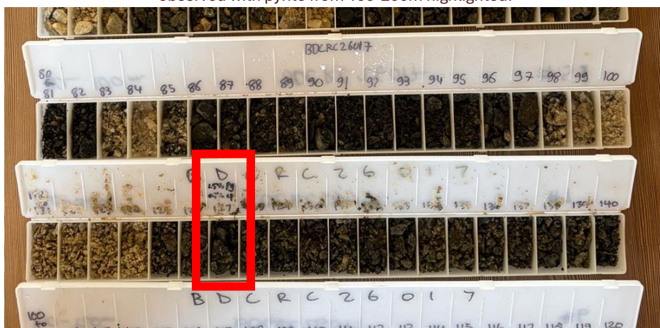
Representative RC rock chip samples from drill hole BDCRC26017 (81–120m), with Chalcopryite (~0.5%) observed with 127-128 199-200m highlighted.
