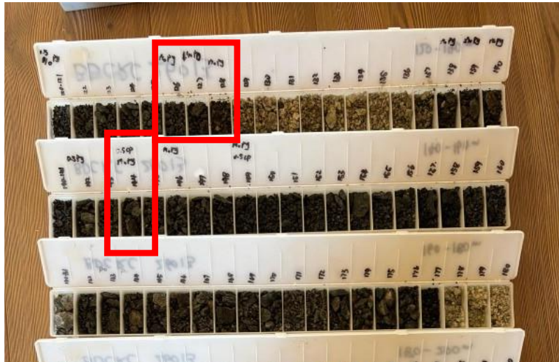
Representative RC rock chip samples from drill hole BDCRC26013 (131–180m), with intersection of Pyrite from 126-128 and Chalcopyrite (~0.5%) observed with pyrite from 229-230m highlighted.
