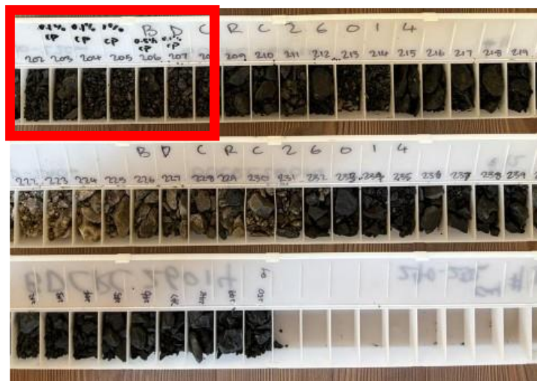
Representative RC rock chip samples from drill hole BDCRC26014 (201–250m EOH), with intersection Chalcopryite (~0.1–0.5%) observed with minor pyrite from 202–207m highlighted.
