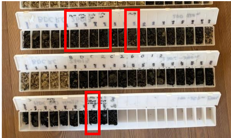
Representative RC rock chip samples from drill hole BDCRC26013 (201–250m EOH), with intersection Chalcopyrite (~0.1–1%) observed with minor pyrite from 206–209m, Chalcopyrite (~1%) observed from 212–213m and Chalcopyrite (~0.5%) observed with pyrite from 247–248m highlighted.
