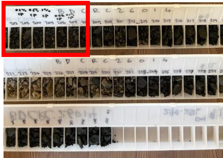
Representative RC rock chip samples from drill hole BDCRC26014 (201–250m EOH), with intersection Chalcopyrite (~0.1–0.5%) observed with minor pyrite from 202–207m highlighted.
